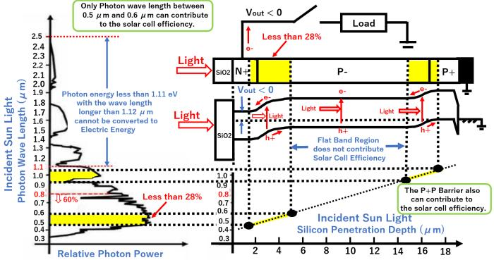
Since the band gap of silicon crystal is 1.1 eV, any photon with the energy greater than 1.1 eV can generate the photo electron and hole pairs. However, without any Barrier Electric field, the photo pairs would recombine themselves and the photo pairs do not contribute to the Solar Cell Efficiency.
