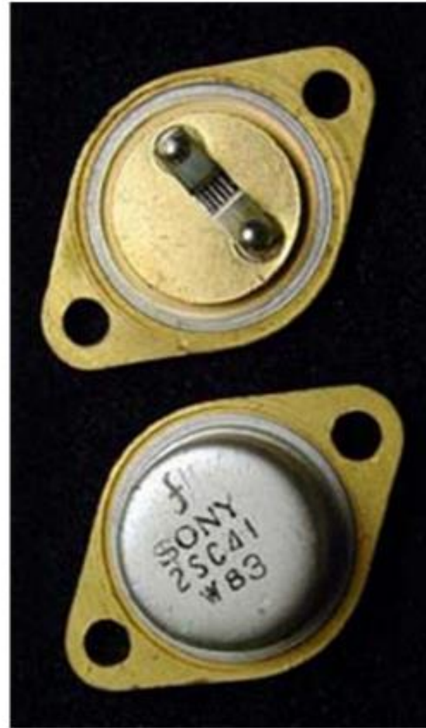
Silicon Power Transistor 2SC41 , Dec 1959
