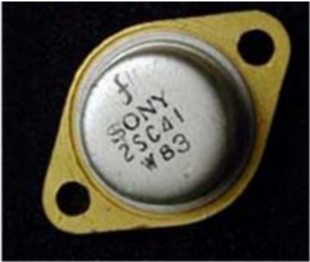
Silicon Power Transistor 2SC41 , Dec 1959
