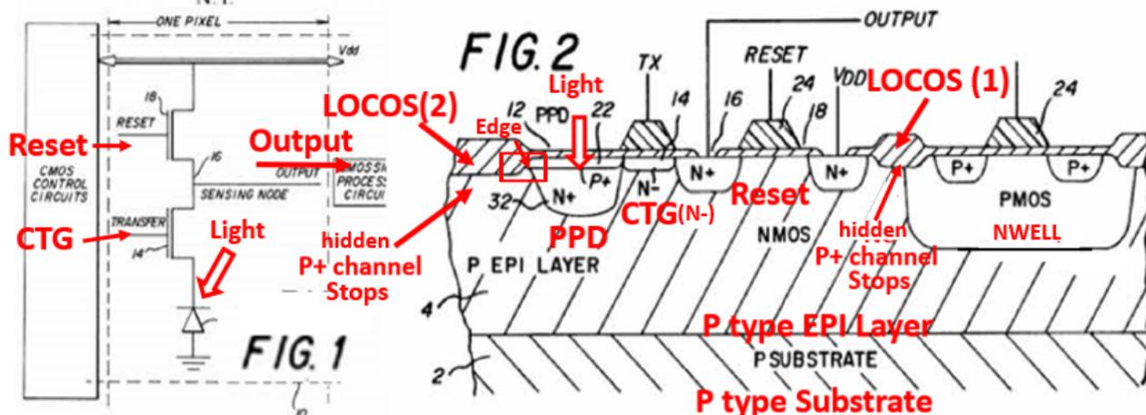
Kodak still used the LOCOS technology for the image sensor process. Yes, there is possibly hidden P+ channel stops for pinning under the **LOCOS (1)** Area Edge and also at the boundary **LOCOS (2)**.
