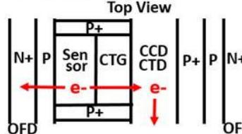
Type(C) Vertical OFD (VOD) PPD with CCD type CTD
