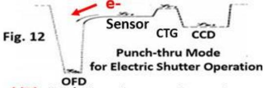
The electric shutter clocking scheme with the complete signal charge draining of no image lag can be achieved by the OFD punch-thru voltage control for any photodiodes, including not only the type (A) of the conventional CCD/MOS photo capacitor but also (B), (C) and (D) type Pinned Photodiodes.
