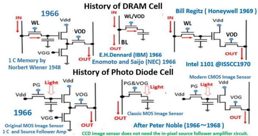
CMOS Inverter and Source Follower circuits are basics for digital circuit design. But we had to wait, till the advancement of CMOS process scaling rule, in order to place the source follower active circuit in each small picture cell area. Meanwhile CCD had a great role in the advancement of image sensors in 1980s. For modern high definition TV image sensor applications, CCD has the power issue and also the limit in charge transfer efficiency of 99.999%, which is not enough now.
