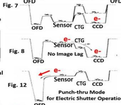
The electric shutter clocking scheme with the complete signal charge draining of no image lag can be achieved by the OFD punch-thru voltage control for any photodiodes, including not only the type (A) of the conventional CCD/MOS photo capacitor but also (B), (C) and (D) type Pinned Photodiodes.
