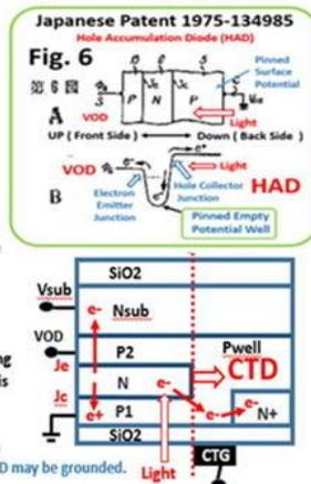
Most CCD Image sensors and CMOS Image sensors today are applied with the combination of the vertical overflow drain (VOD) and Pinned Photodiode.
