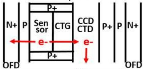
**Type(C) Vertical OFD (VOD) PPD with CCD type CTD**
