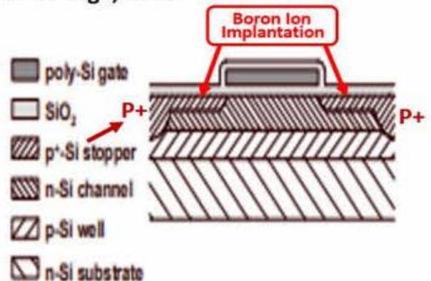
Figure 3. Cross section of a buried-channel CCD on n-Si substrate including light windows and pinned interface potential in the non-covered CCD channels (the cross section is made perpendicular to the CCD channel).
