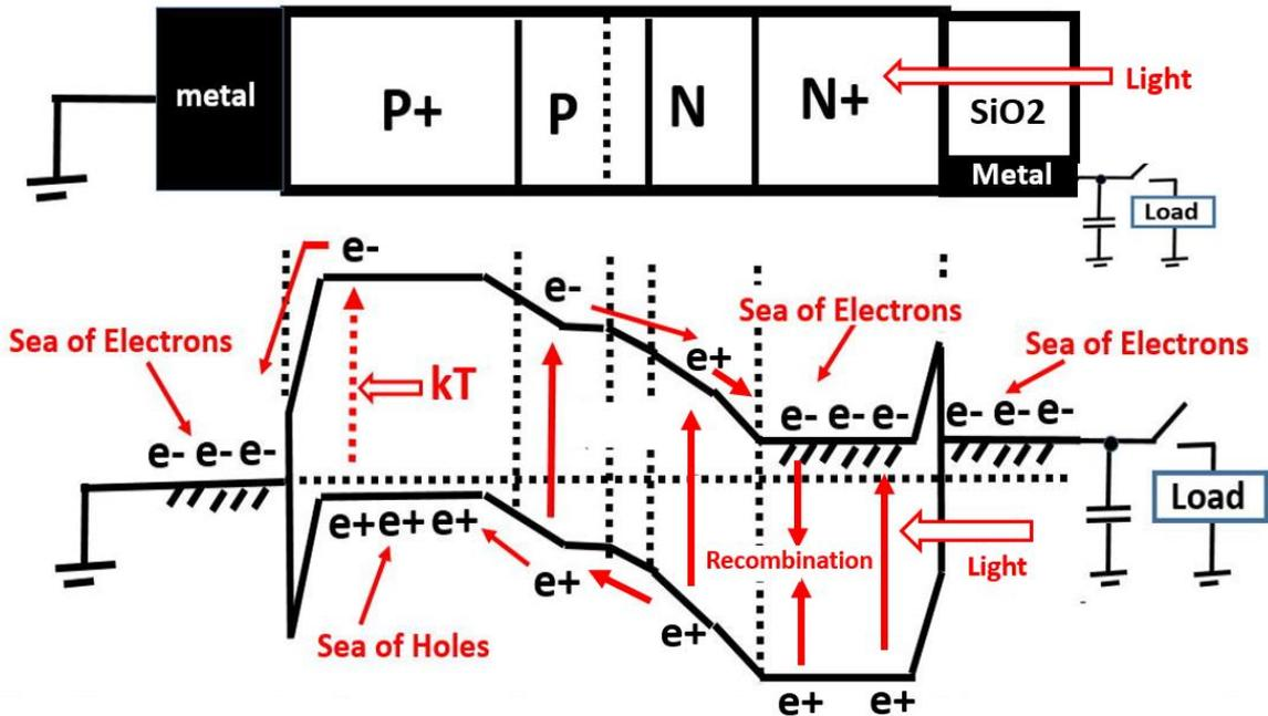
Pinned Photodiode (PPD) has the excellent short wave blue light sensitivity, the very low surface dark leakage current feature and the complete charge transfer capability for the excellent image lag free picture quality needed for the electric shutter. Now this double junction type PPD is proposed to apply for solar cells.
