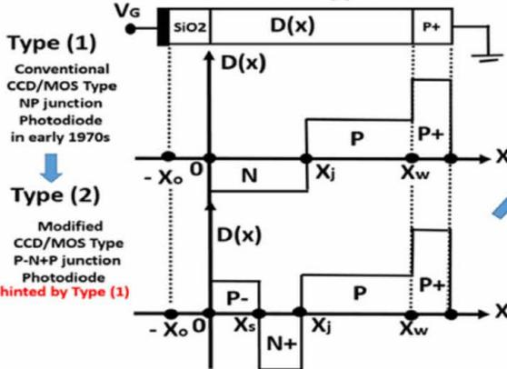
**Pinned Photodiode proposed in 1975**
