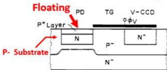
Fig.5. P+NP- structure photodiode
