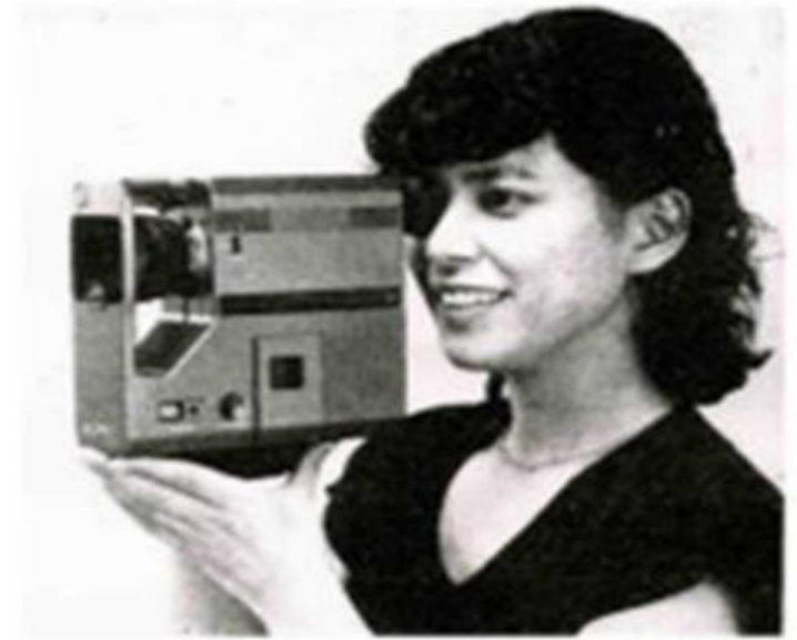
Sony 1980 Video Movie has in one body an 8 mm VTR and One Chip FT CCD Image Sensor with the PNP Double Junction type Pinned Photodiode developed by Hagiwara in 1978
