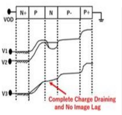
JPA1975-134985 with In-Pixel Vertical Overflow Drain (VOD)
