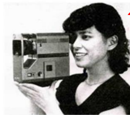
Sony 1980 Video Movie has in one body an 8 mm VTR and One Chip FT CCD Image Sensor with the PNP Double Junction type Pinned Photodiode developed by Hagiwara in 1978
