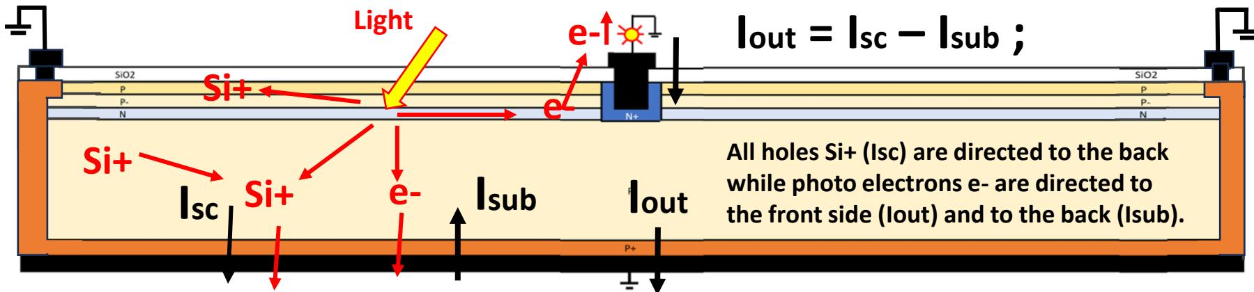
Electrons are guided swiftly toward the center N+ outlet region by the voltage drop  $V_1 > 0$ .
