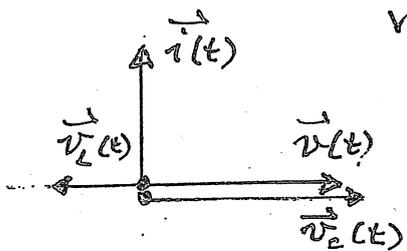
$$\left\{ \begin{aligned} \vec{v}_C &= 1.1 \vec{v}(t) \\ \vec{v}_L &= -0.1 \vec{v}(t) \\ \vec{i}(t) &= \frac{1}{\vec{Z}} \vec{v}(t) = \frac{j}{100} \vec{v}(t) \end{aligned} \right.$$
