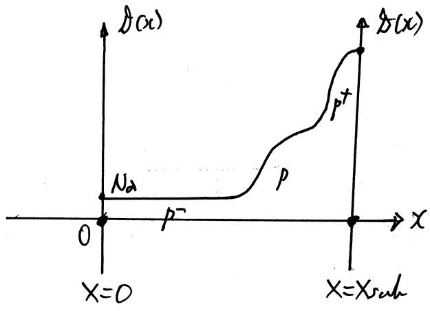
$$\begin{aligned}\phi(0) &= kT \ln \left( \frac{N_{dd}}{N_A} \right) \\ \phi(X_{sub}) &= 0\end{aligned}$$
