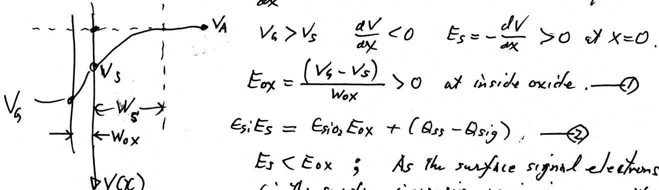
$E_s < E_{ox}$ ; As the surface signal electrons  $Q_{sig}$  (in the surface inversion region increased the surface electric field  $E_s$  and the surface potential both decrease.)
