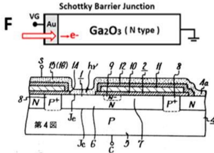
Fig. 6: Cross sectional view of Type F Schottky barrier photo sensor.
