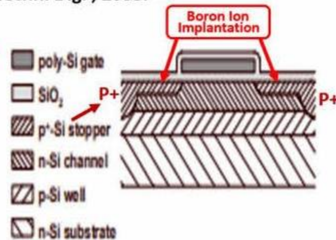
Figure 3. Cross section of a buried-channel CCD on n-Si substrate including light windows and pinned interface potential in the non-covered CCD channels (the cross section is made perpendicular to the CCD channel).
