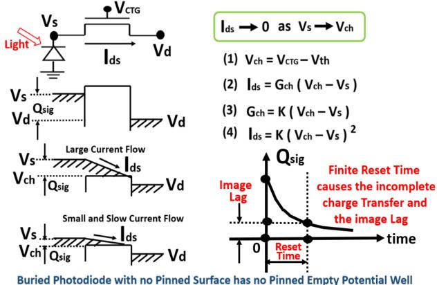
while Pinned Photodiode with no Pinned Surface has no Pinned Empty Potential Well
