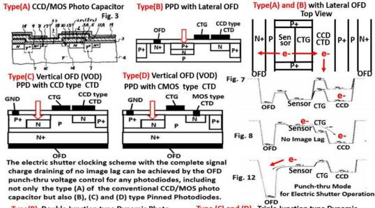
Type (C) and (D) Triple Junction type Dynamic Type(B) Double Junction type Dynamic Photo Transistor (PPD) invented in 1975 by Hagiwara. Photo Thyristor (HAD) invented in 1975 by Hagiwara
