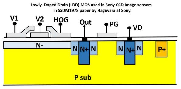
For ONE chip Image sensor in NTSC system, Sony(Hagiwara) needed the CCD clock frequency of 14.31818 MHz. Sony (Haiwara) used the thermal diffusion N+ for the metal contact with the lightly doped drain for the prcharge (PG) gate.
