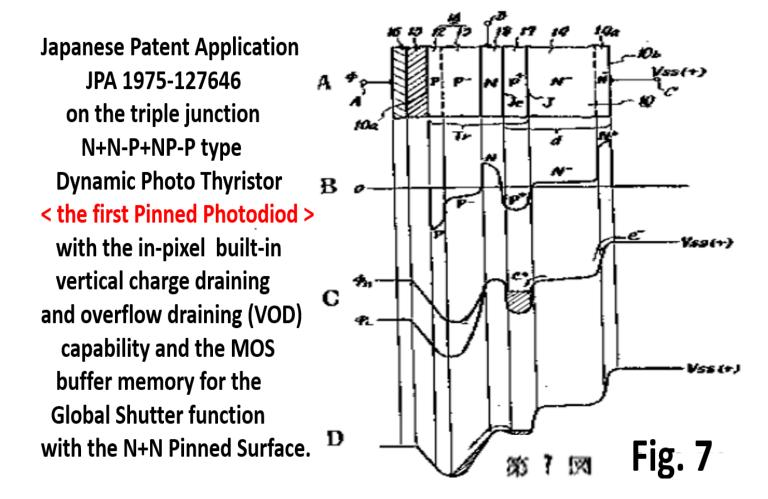
It is well known that the short wave blue light cannot penetrate more than 0.2  $\mu$ m in depth into the silicon crystal. However, the surface N+N barrier electric field can be created at the silicon surface within the 0.2  $\mu$ m in depth and can be used effectively to separate photo electron and hole pairs generated in the vicinity of the Si surface.
