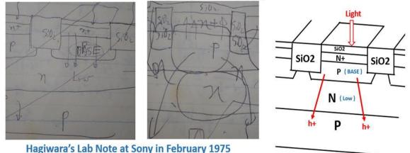
In 1975 at Sony, Yoshiaki Hagiwara filed three Japanese patents JPA1975-127646, JPA1975-127647 and JPA1975-134985 on the Pinned Surface Photodiode with the VOD function which is later called as Sony Hole Accumulation Diode (HAD). Hagiwara did not file a patent on the SiO2 device isolation but this lab note shows that Hagiwara had an idea of forming the Shallow Trench Isolation by the Local Oxidation Method, which was hinted by the LOCOS isolation in 1970s.
