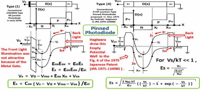
The surface electric field Es of the P+NP junction type Pinned Photodiode is also very large which is worse since the surface electric field depends also on the surface P+ doping level Npp. Type (2) and Type (3) modifications may help reducing the surface electric field Es.
