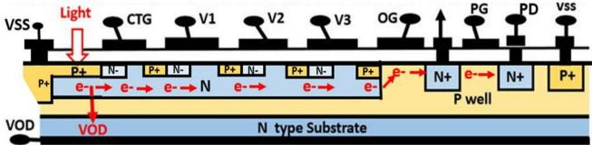
The electric shutter function becomes possible only in the CCD/MOS type photo capacitor sensor and Pinned Photodiode (PPD), both of which have the complete charge transfer capability of no image lag. However, Buried Photodiode (BPD) is not always Pinned Photodiode (PPD). But, Pinned Photodiode (PPD) is always Buried Photodiode (BPD). Buried Photodiode (BPD) and Pinned Photodiode (PPD) are both the same double junction type PNP dynamic photo transistors invented by Yoshiaki Hagiwara in 1975.
