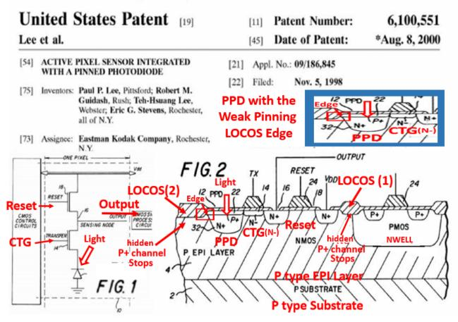
Kodak still used the LOCOS technology for the image sensor process. Yes, there is possibly hidden P+ channel stops for pinning under the LOCOS (1) Area Edge and also at the boundary LOCOS (2).
