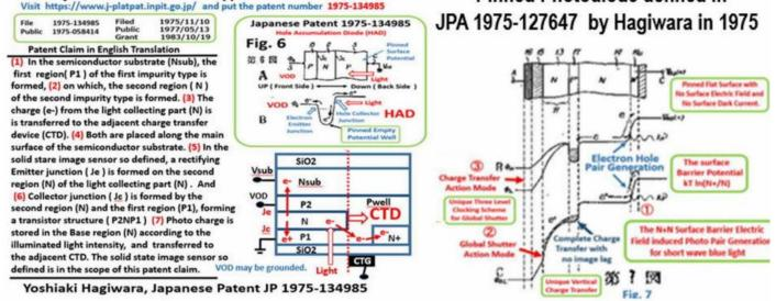
Hagiwara applied two Japanese Patents JPA1975-127646, and JPA1975-127647 for the back light illumination type Pinned Photodiode with Global Shutter Function which is a very important feature needed for the modern CMOS image sensors. The complete charge transfer mode and the no image lag feature is also shown and implied by the empty potential well of the buried charge storage region.
