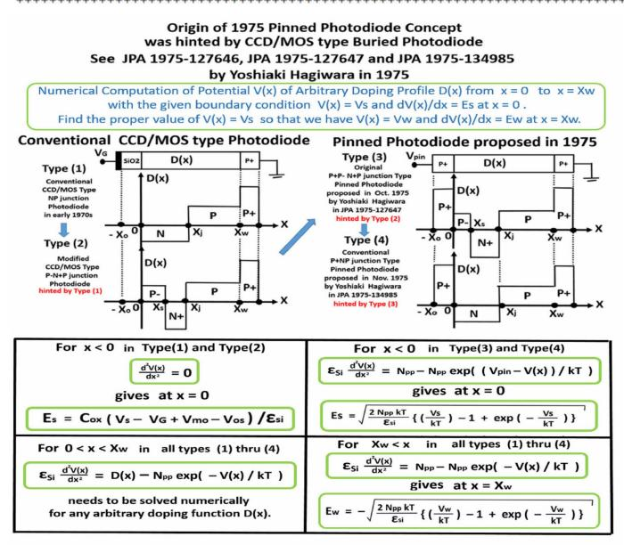
The conventional Buried Channel CCD/MOS type photodiode has a very large surface electric field Es.
