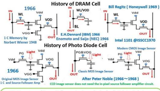
CMOS Inverter and Source Follower circuits are basics for digital circuit design. But we had to wait, till the advancement of CMOS process scaling rule, in order to place the source follower active circuit in each small picture cell area. Meanwhile CCD had a great role in the advancement of image sensors in 1980s. For modern high definition TV image sensor applications, CCD has the power issue and also the limit in charge transfer efficiency of 99.999%, which is not enough now.
