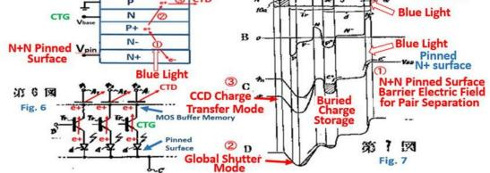
Global Shutter Mode with Built-in MOS Capacitor Buffer Memory Global Shutter Function and the surface N+N doping slope Barrier Electric Field Photo Pair Generation
