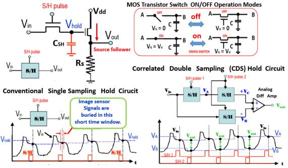
Image sensor Signals are buried in the large clock noises.
