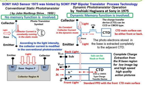
History of dynamic Solid State image sensing structure from BCCD type MOS capacitor to the P+NPN junction Pinned Photodiode capacitor
