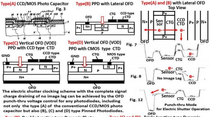
**Type(B)** Double Junction type Dynamic Photo Transistor (PPD) invented in 1975 by Hagiwara. Type (C) and (D) Triple Junction type Dynamic Photo Thyristor (HAD) invented in 1975 by Hagiwara
