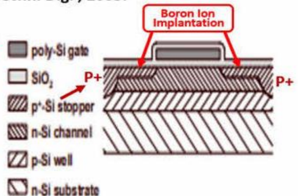
Figure 3. Cross section of a buried-channel CCD on n-Si substrate including light windows and pinned interface potential in the non-covered CCD channels (the cross section is made perpendicular to the CCD channel).
