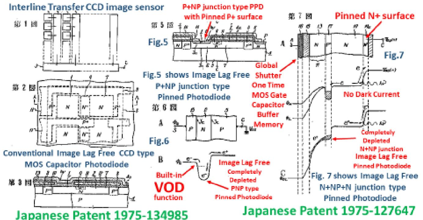
With the pinned window and the pinned surface potential, when the PPD is completely depleted of signal charge, the empty potential well of the collection region is also pinned to a certain voltage that can be designed properly by adjusting the impurity doping profile of the P+NP junction structure of the PPD.
