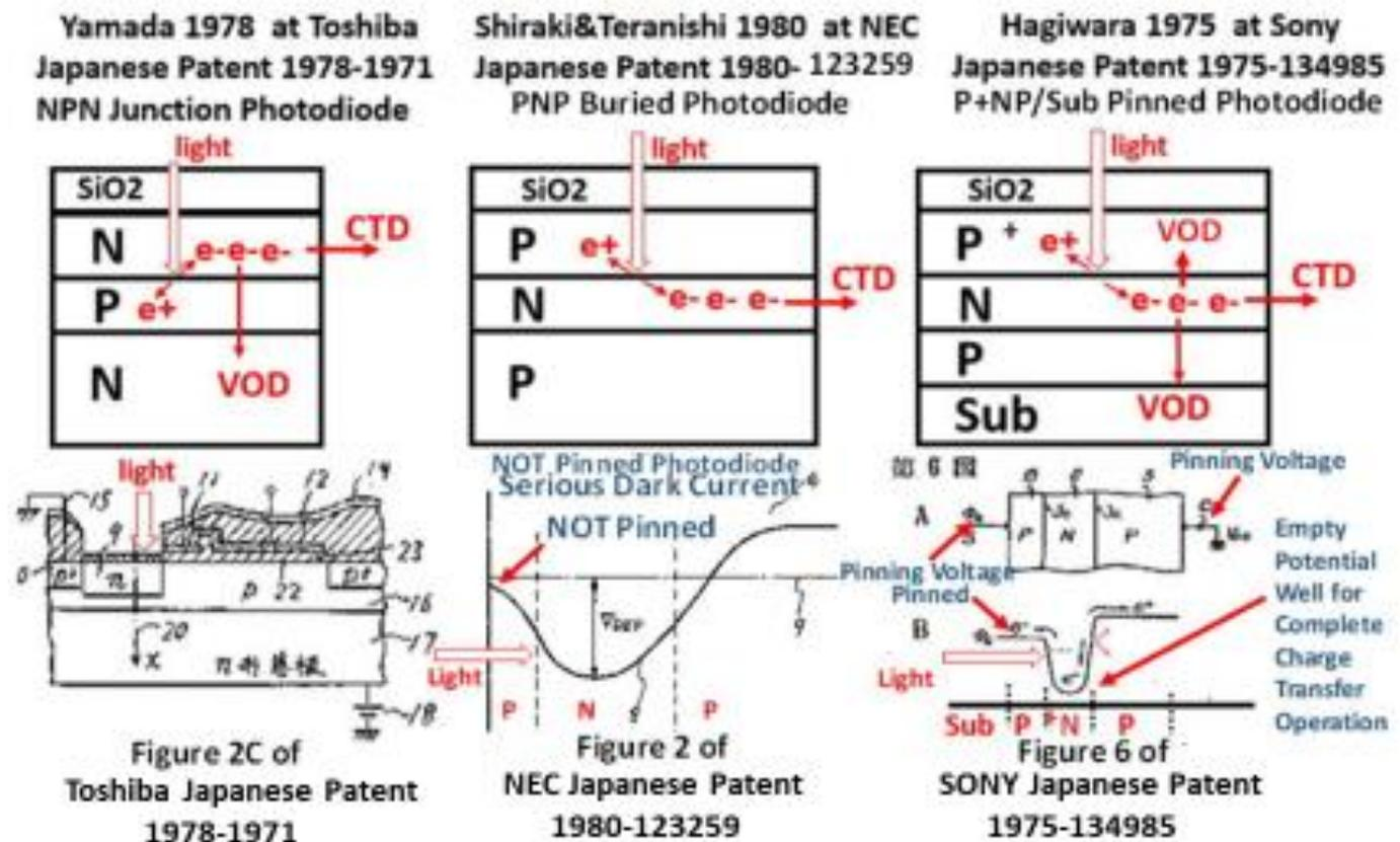
Depleted Buried Photodiode (DBPD) is designed to have the signal charge collection region deplete out when reset. The signal charge is to be transferred to the adjacent charge transfer device (CTD) thru a charge transfer gate (CTG) with the CCD-like complete charge transfer operation mode, resulting image lag free picture quality. The CTG is a by-pass gate, normally not used as a buffer memory.
