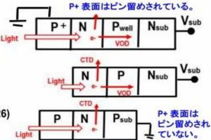
Comparison of Various Light Detecting Photo Sensor Structures
