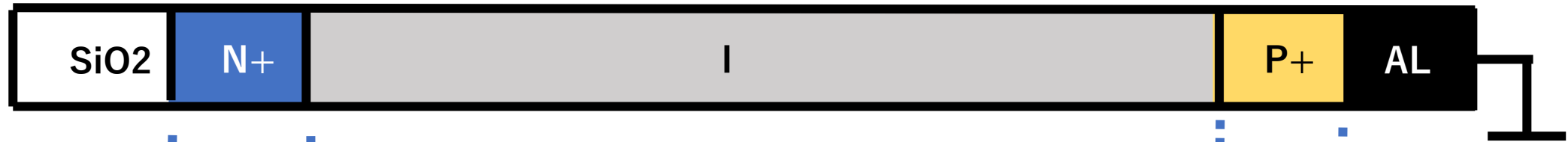
(a) Floating-Surface P-I-N Single Junction type Solar Cell
