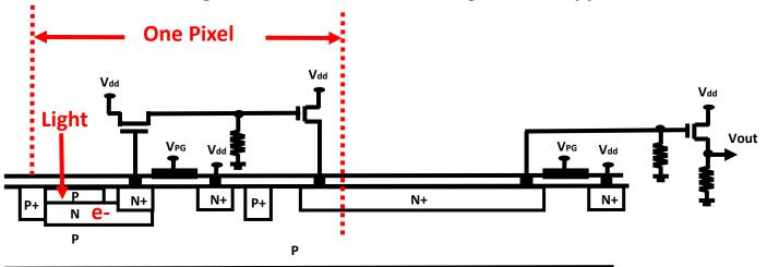
Solar Cells do not need the source-follower current- amplifier used in CMOS image sensors nor the CCD type charge transfer device itself. The completely depleted N- region of the P+P-N-P-P+ double junction type Solar Cell shown below has a long empty potential well acting as a free space for photo electrons, being drained to the small outlet N+ region.
