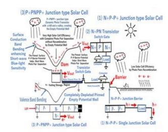
Fig. 2 Water Barrier, Water Gate and Water Dam Analogy of Semiconductor.
