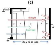
Short-wave blue-light cannot penetrate more than 0.1  $\mu$  m in depth at the silicon crystal surface.
